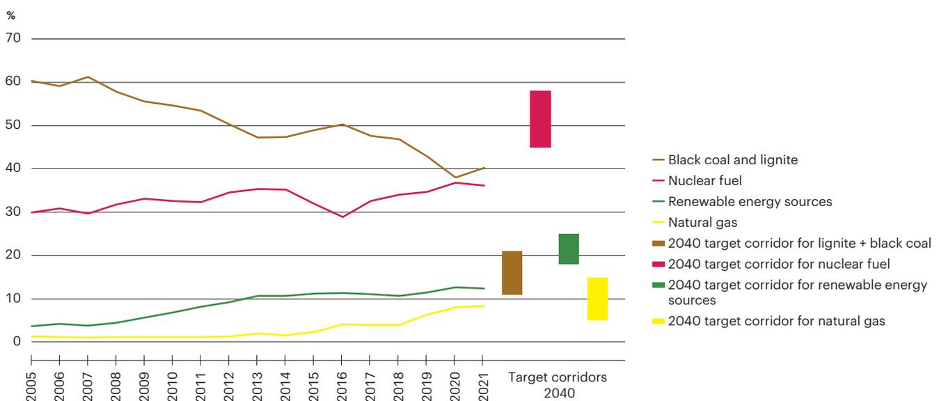
The target corridors for each source (nuclear 46%–58%, renewables and secondary sources 18%–25%, natural gas 5%–15%, lignite and black coal 11%–21%) are plotted in the right-hand side of the graph in the corresponding colours.
