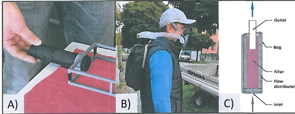
Fig. 1: A) cartridge frame before wrapping with fleece polyester knit, B) filter set, C) diagram of the filter cartridge in the backpack
