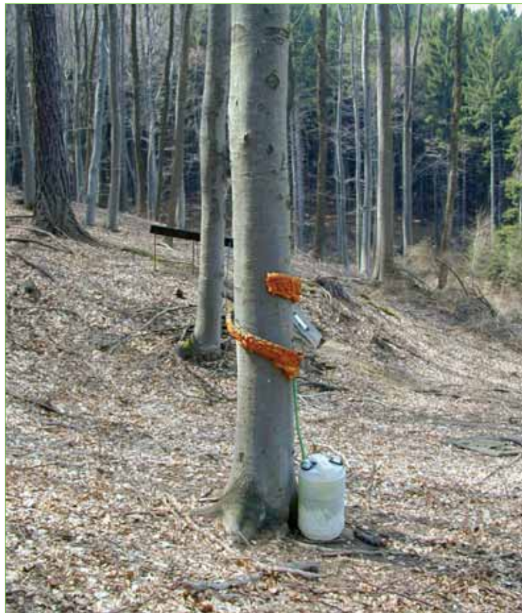
Obr. 5.2.9.4 Stok po kmeni Stemflow measurement
