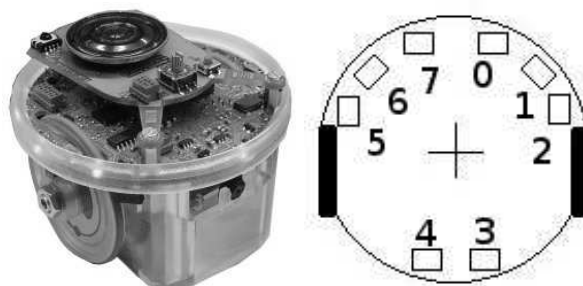
Figure 1: Miniature e-puck robot has eight infrared sensors and two motors.
