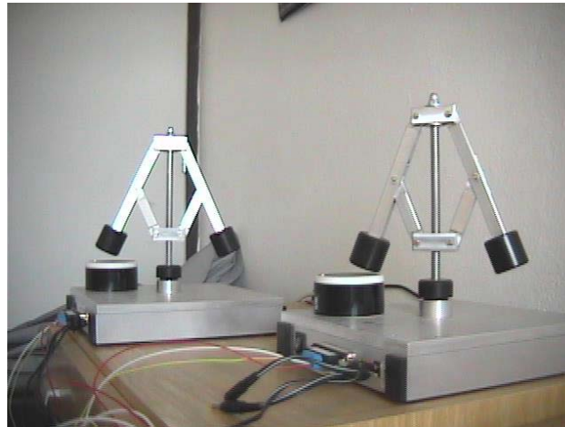
Fig. 5: The snapshot from IP camera of the two models of Watt's regulator
