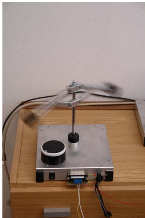
Figure 1: The model of Watt's governor
