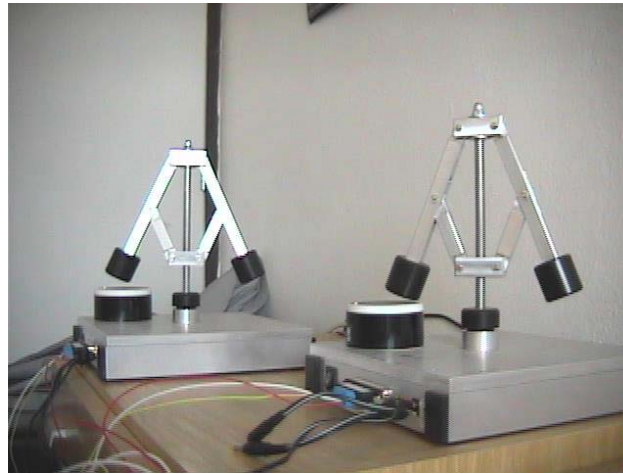
Fig. 5: The snapshot from IP camera of the two models of Watt's regulator
