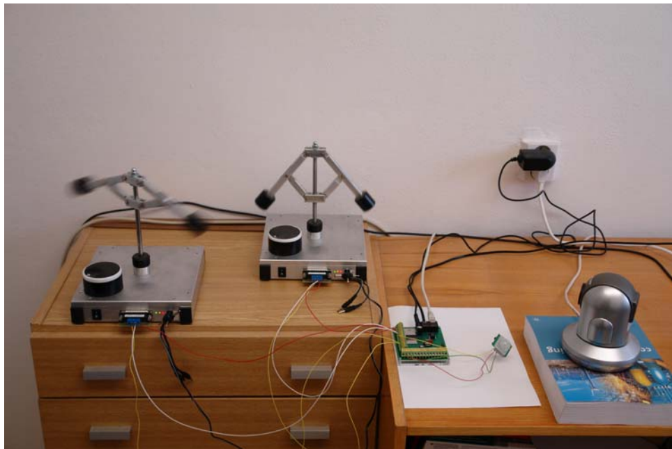
Fig. 4: The linking of two models of Watt's regulator with the web processor CTRL V4
