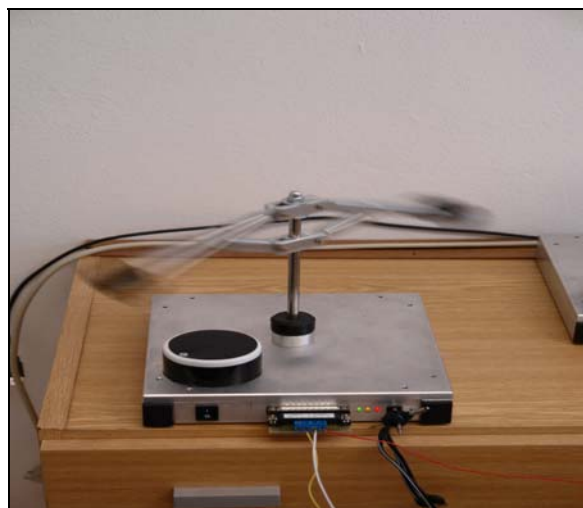
Figure 4: The electromechanical model of Watt's regulator (source: the author).
