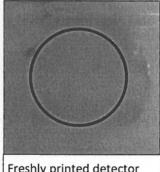
Freshly printed detector point from both side of a foil.
