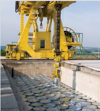
The waste drums are placed within the vaults by a gantry crane; the operator's cabin is shielded to protect the operator from radiation exposure.
