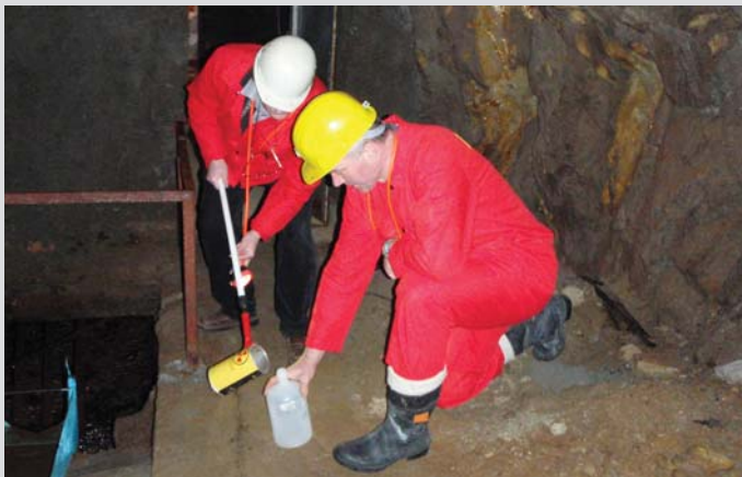
Sampling of water to be subjected to analysis in accordance with approved monitoring programmes for the Bratrství repository.
