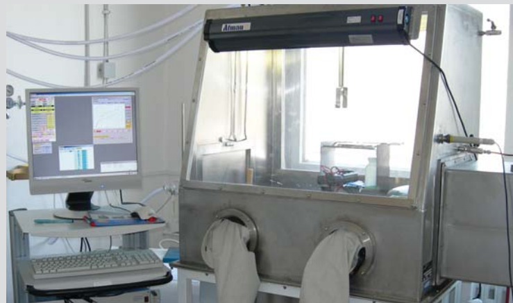
Experimental equipment for studying electrochemical characteristics at the Nuclear Research Institute at Řež – nickel electrolyser installed in dry box.
