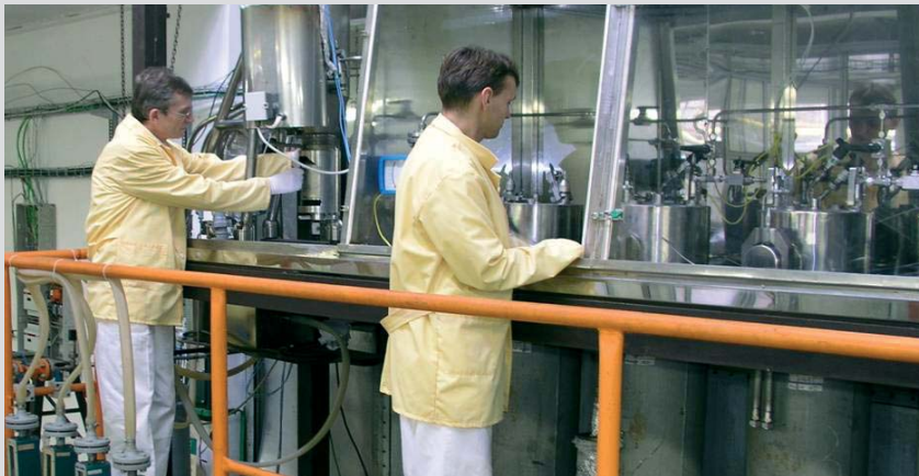
Experimental line for the fraction distillation of fluorides (Nuclear Research Institute, Řež). This method allows certain components of spent nuclear fuel to be separated.
