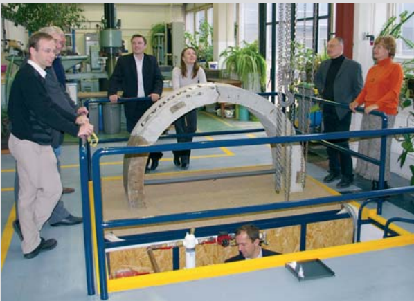
Launch of an experiment carried out as part of the Euroatom TIMODAZ project at a laboratory at the Centre for Experimental Geotechnics of the Czech Technical University in Prague. The aim of the experiment is to study the impact of long-term thermal load on tunnel lining stability.
