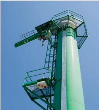
Crane used for transport package drop tests.
