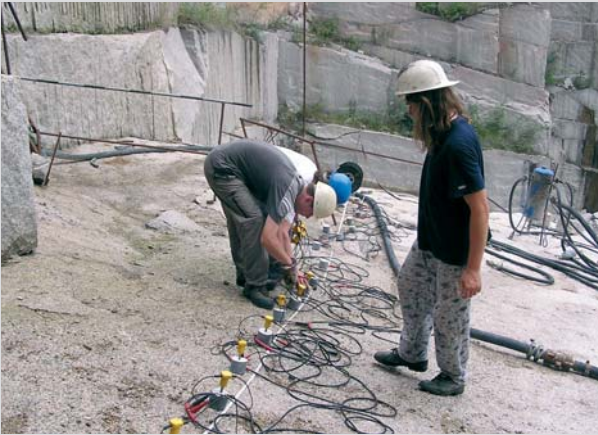
Assessment of the impact of tunnelling on granitoid rock based on the study of physical conditions in the surroundings of open quarries - work in the Ruprechtice quarry, northern Bohemia.
