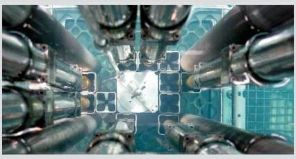
Preparation of the active zone for a basic critical experiment to be carried out in the "Vrabec" educational reactor at the Faculty of Nuclear Sciences and Physical Engineering of the Czech Technical University in Prague. The active zone comprises a module containing fluoride salts.
