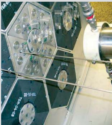
Preparation for the measurement of the neutron field in a model of part of the transmuter under development with fluoride salt-based fuel. The target chamber of the neutron source can be seen on the right-hand side of the photograph.
