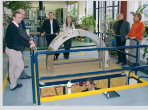
Launch of an experiment carried out as part of the Euroatom TIMODAZ project at a laboratory at the Centre for Experimental Geotechnics of the Czech Technical University in Prague. The aim of the experiment is to study the impact of long-term thermal load on tunnel lining stability. Assessment of the impact of tunnelling on granitoid rock based on the study of physical conditions in the surroundings of open quarries - work in the Ruprechtice quarry, northern Bohemia.
