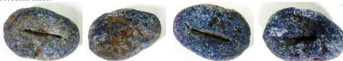
Figure 9. Medieval glass bead before (left) and after plasma treatment (right).
