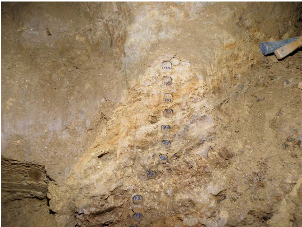
Figure 4 Plastic boxes for paleomagnetic samples within the profile, Hermannshöhle, Teichkluft. Numbers means distance in centimeters from profile bottom (photo by P. Bosák)
