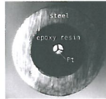
Figure 2. The three-segment probe (magnified front view).
