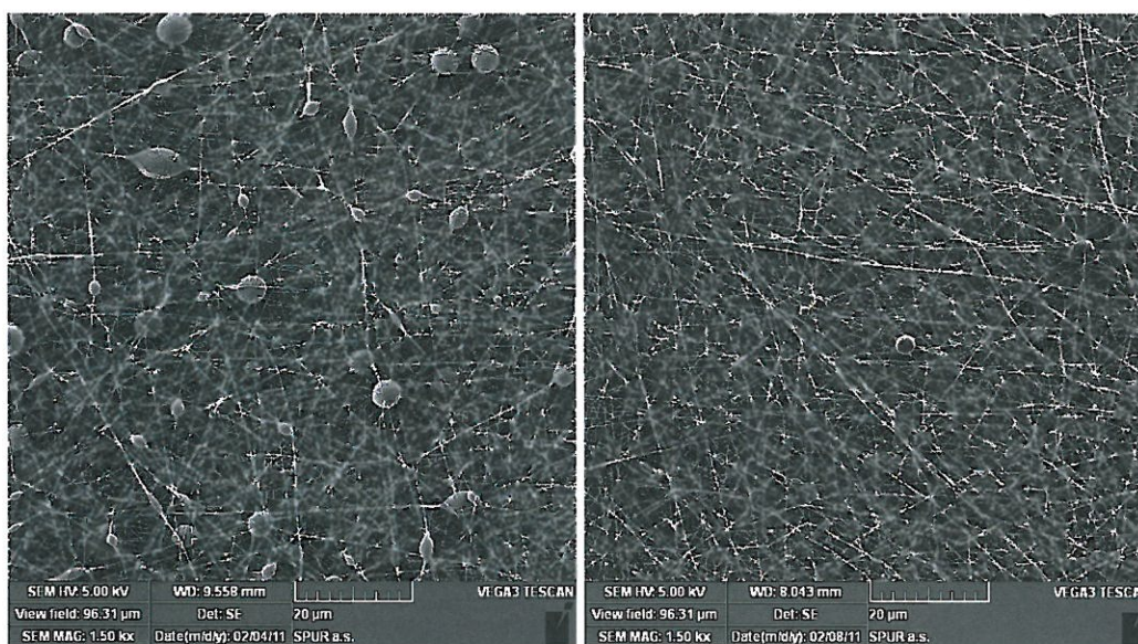
FIGURE 9. Nanostructure formed without any additives, magnification 1 500×.
