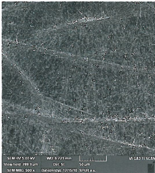
FIGURE 3. Accumulation of PU nanofibres around conductive microfibres of a spunbond support, magnification 500×.
