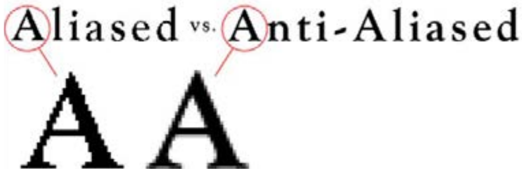
Figure 8: Comparison of an uppercase “A”, aliased and anti-aliased.
