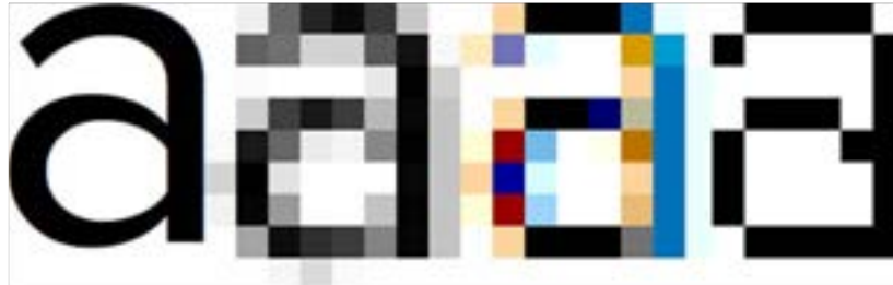
Figure 7: Rendering of a lowercase “a” by three different rendering engines.
