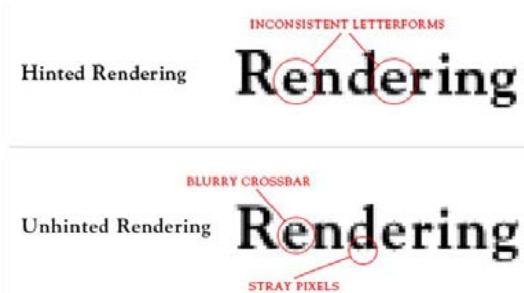
Figure 9: Visual comparison of differences between hinted and unhinted rendering of a typeface.
