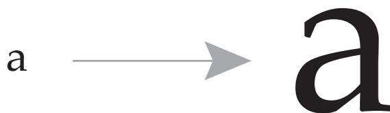
Figure 6: A font stored in Bézier curves does not show any distortion when enlarged.
