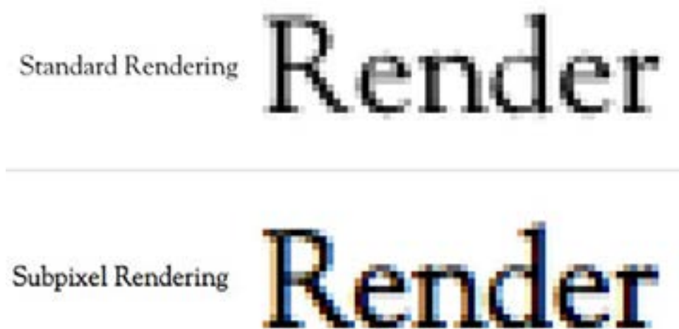
Figure 10: Standard rendering causes greyscale pixels to be added, while subpixel rendering creates pixels of different colour shades.
